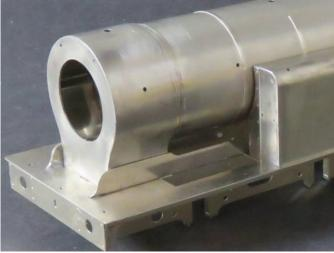
78) Fit Buffer Bases to the buffer beams.
