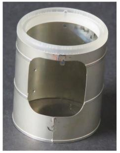
65) Offer to both plastic rings, in the picture adjacent the smokebox end is on the right should fit into (P53) pictured on previous page, study all pictures carefully. Do not force the metal boiler into the plastic, if it is too big take off the elastic bands and evenly file off a small amount from the jointing edges, repeat until it is a snug fit. When
